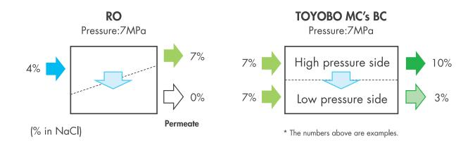
The same or similar concentrated solutions are applied to both shell side and bore side and a certain pressure is applied to one side, the same osmotic pressure difference as applied hydraulic pressure can be obtained
