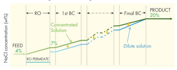
Lower concentration gap between inlets of both sides enables you to achieve 20% NaCl with minimum energy inputs using only one high pressure pump
