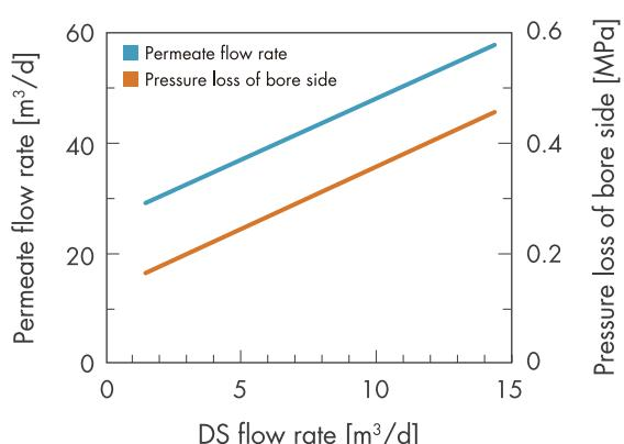
\*Pressure on bore side should be lower than pressure on shell side
