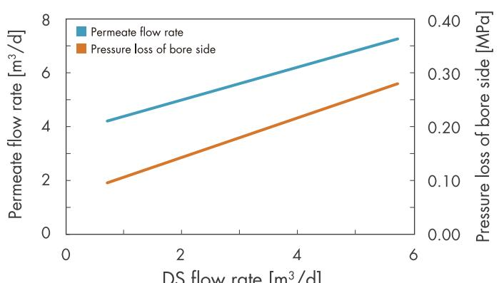
\*Pressure on bore side should be lower than pressure on shell side
