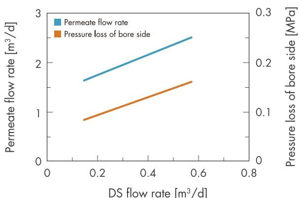
\*Pressure on bore side should be lower than pressure on shell side
