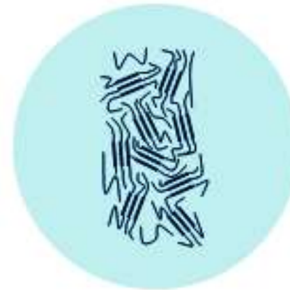
Polyethylene Irregular molecular structure (Low orientation)
