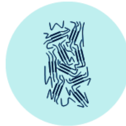
Polyethylene Irregular molecular structure (Low orientation)
