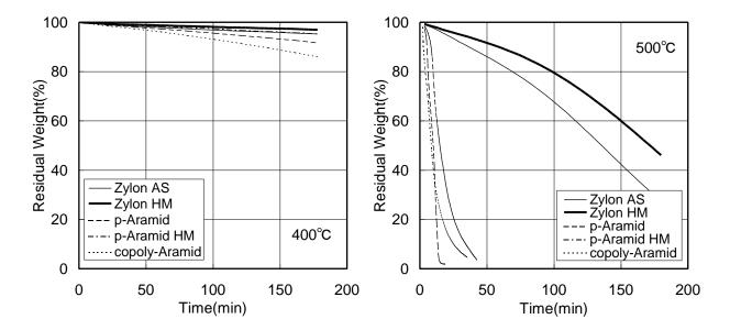
**<u>5.3 Strength retention after thermal treatment</u>** These figures show the effect of thermal treatment in air on residual strength. ZYLON<sup>®</sup>HM shows a little higher heat resistance than ZYLON<sup>®</sup>AS.
