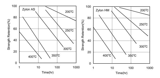
Strength retention after thermal treatment is compared with Aramid fibers at several temperatures.
