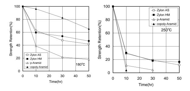
The strength of ZYLON<sup>®</sup> gradually decreases even at the temperature of less than 100°C in high humidity condition. ZYLON<sup>®</sup> fiber should be stored free from high humidity at normal room temperatures.
