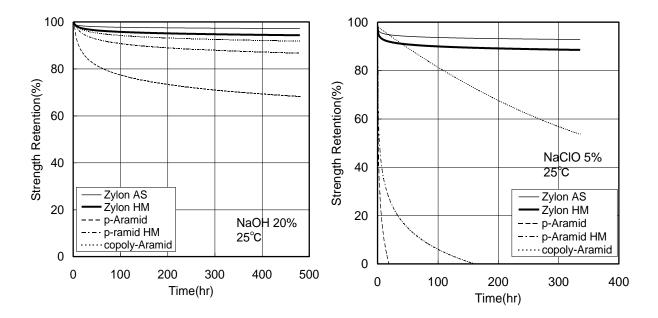
At higher temperatures, the strength of ZYLON<sup>®</sup> AS staple fiber decreases in acid and also in alkaline.
