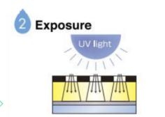
Expose the plate through the negative film to UV light having 360 nm wave length. Determine the correct exposure time using a 21 steps grey scale. Follow "TIPS FOR Printight®" in each case.
