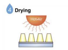
Dry the plate in a hot-air dryer after taking-off the surface water with a sponge roll. Drying time depends on the type of the plate. Follow "TIPS FOR Printight®" in each case.
