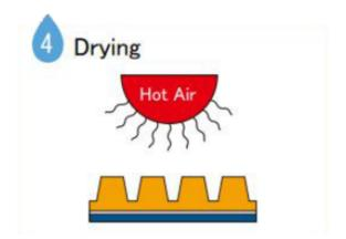
Dry the plate in hot-air dryer after taking-off the surface water with sponge roll.
