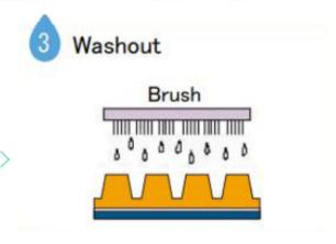
Washout exposed plate with water. Use the special washout machine suitable for TOYOBO PRINTIGHT®
