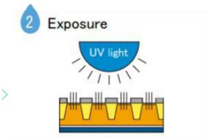
Expose plate to UV light having 360nm wave lengths.
