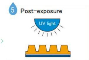
Expose the developed plate after drying again to UV light in order to get stability. Post exposure time.
