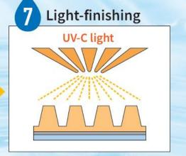
Expose to UV-C light to eliminate a plate tackiness.
