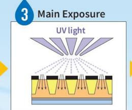
Expose to UV light with 360nm wave lengths.
