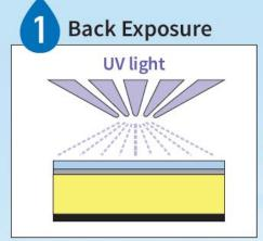
Expose to UV light from the back side to establish floor.
