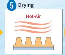
Remove water droplets from a plate surface, and dry it in a hot-air dryer.
