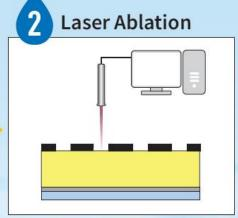
Depict images through an IR laser head to a laser ablation layer directly.
