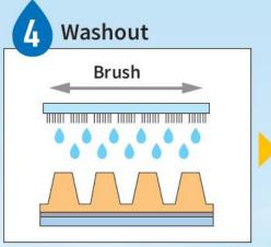
Wash out with tap water and a small amount of mild detergent. Use washout machines for Cosmolight™.
