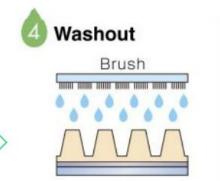
Remove the negative film and process the plate in Cosmolight® washout unit.
