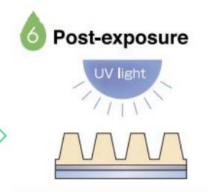
Expose to UV light again to complete photo-curing.
