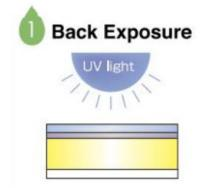
Expose to UV light through substrate film on back side of plate.
