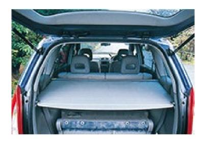
Based on polyester spunbond nonwoven fabric technology, it is a light and durable leather-like nonwoven fabric with breathability. It is mainly used as a tonneau cover material for automobiles taking advantage of its light weight and eco-friendly features.
